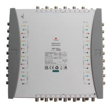
Cascade multiswitch for 4 Satellite positions with 17 inputs and 17 trunk outputs, suitable for distributing satellite and terrestrial signals in small to large sized systems. Available with 24 subscriber outputs and powered by the TMS PSU external power supply either directly or via the SAT trunk lines.
