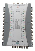
Cascade multiswitch for 4 Satellite positions with 17 inputs and 17 trunk outputs, suitable for distributing satellite and terrestrial signals in small to large sized systems. Available with 12 subscriber outputs and powered by the TMS PSU external power supply either directly or via the SAT trunk lines.
