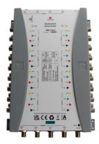
Cascade multiswitch for 4 Satellite positions with 17 inputs and 17 trunk outputs, suitable for distributing satellite and terrestrial signals in small to large sized systems. Available with 8 subscriber outputs and powered by the TMS PSU external power supply either directly or via the SAT trunk lines.
