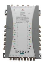
Cascade multiswitch for 3 Satellite positions with 13 inputs and 13 trunk outputs, suitable for distributing satellite and terrestrial signals in small to large sized systems. Available with 16 subscriber outputs and powered by the TMS PSU external power supply either directly or via the SAT trunk lines.
