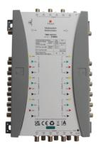
Cascade multiswitch for 3 Satellite positions with 13 inputs and 13 trunk outputs, suitable for distributing satellite and terrestrial signals in small to large sized systems. Available with 12 subscriber outputs and powered by the TMS PSU external power supply either directly or via the SAT trunk lines.
