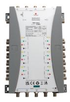
Cascade multiswitch for 3 Satellite positions with 13 inputs and 13 trunk outputs, suitable for distributing satellite and terrestrial signals in small to large sized systems. Available with 8 subscriber outputs and powered by the TMS PSU external power supply either directly or via the SAT trunk lines.
